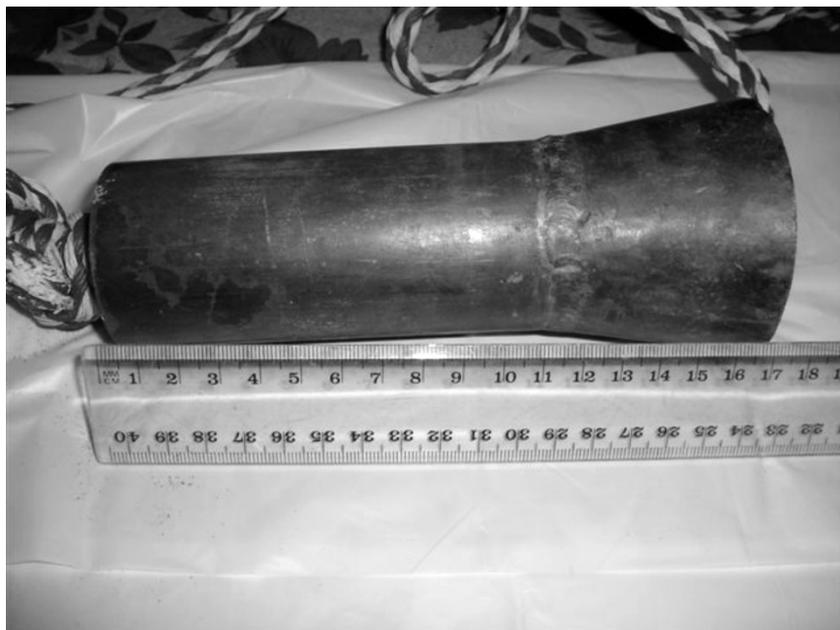
**Figure 1.** The metal scoop used for sampling from sub-tidal sea-grass beds. Opposed to more commonly used meiofauna sampling devices, such as dredges, the robust metal scoop was able to penetrate the dense root web in the sea-grass beds, making it possible to sample this otherwise less accessible habitat
